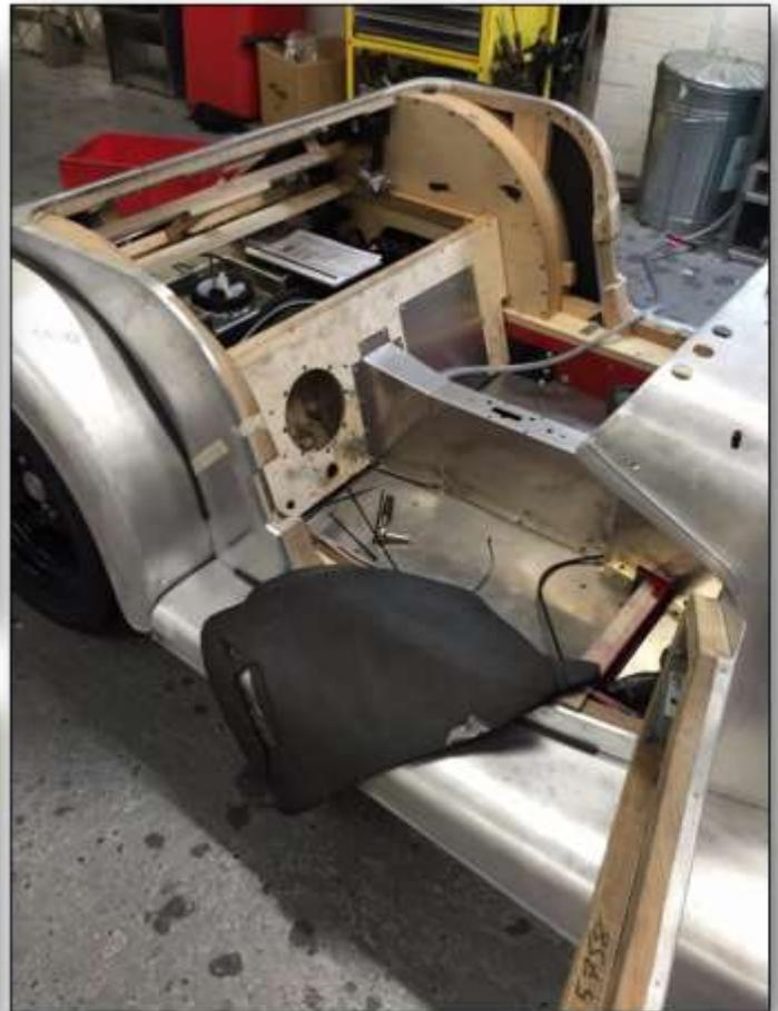
Access Panels through Bulkhead. Note Sheet Metal Floors.
