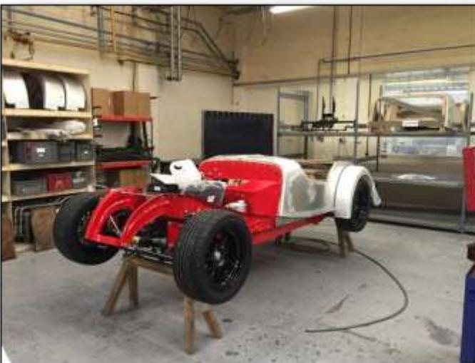
Wide tires necessitate the rear wing width. Red power coating.
