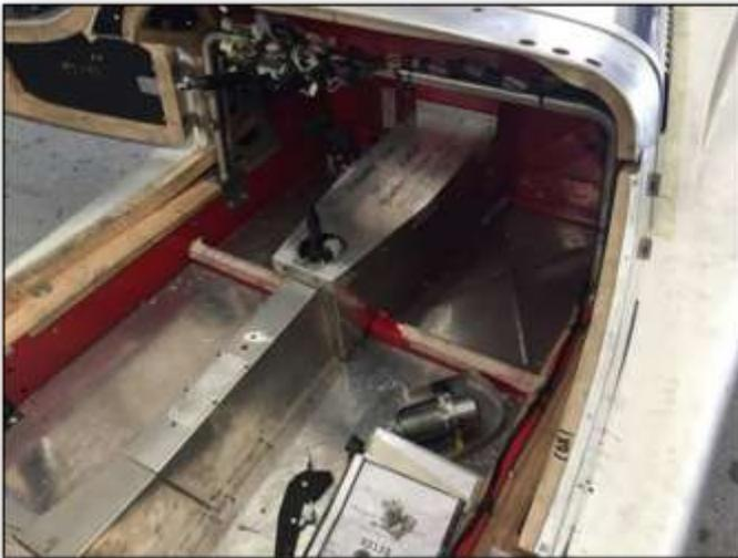
Boxed transmission tunnel and no hand brake evident.
