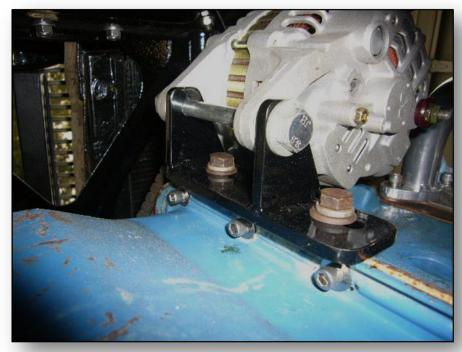
View from below showing the alternator bracket (in black) assembled to the engine.
