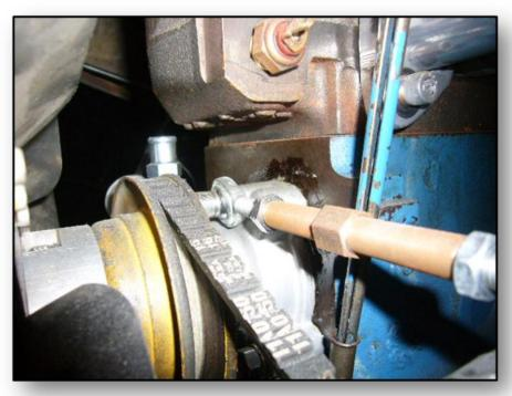
The tensioner in place with the new Vee belt fitted on the pulley.
