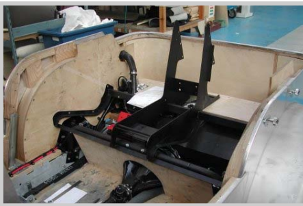
Four Seater Rear Body Contours and Rear Seat Folding Mechanism at Morgan Factory.
