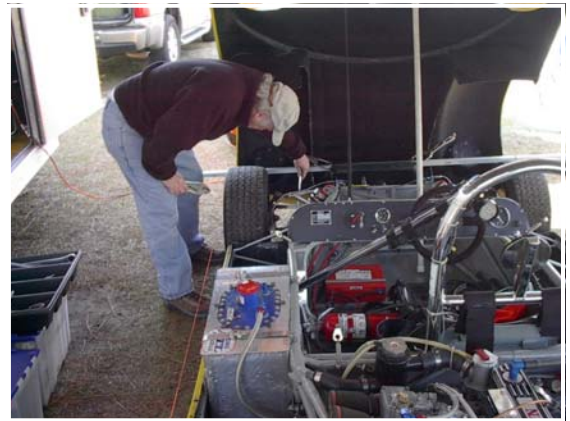
Ray Morgan adjusting the front toe-in on the Merlyn. I thought swerving back and forth was what you were supposed to do?
