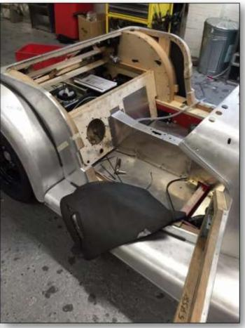
Access Panels through Bulkhead. Note Sheet Metal Floors.
