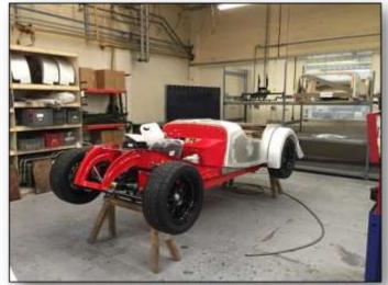
Wide tires necessitate the rear wing width. Red power coating.
