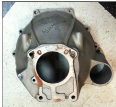
Aluminum bell housing 4/4, with annular hydraulic clutch release.
