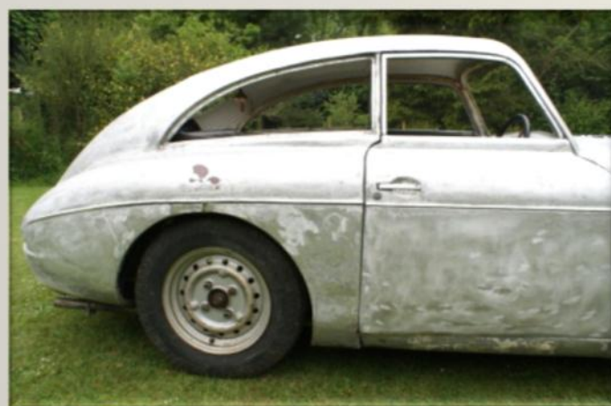
After removing lots of filler and welding the split aluminium body the swage lines and original shape of the Touring styled copy can be seen.
