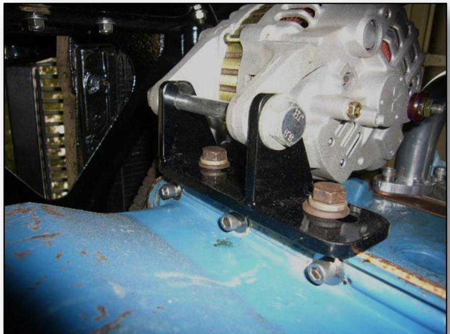
View from below showing the alternator bracket (in black) assembled to the engine.
