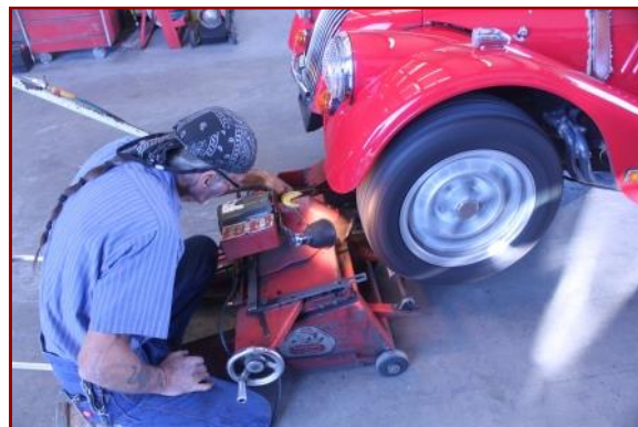
Truing the tires by shaving the rubber to ensure the tire is actually round.
