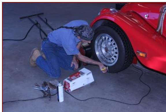
Once the tire is round, balance the wheels on the car. The technician uses a strobe and spins the tire to high speeds to see where the weights should go.
