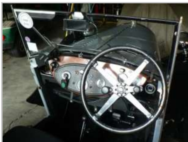
The fuel mixture gage is the modern looking thing on the far right of the dash, visible through the F4's steering wheel.
