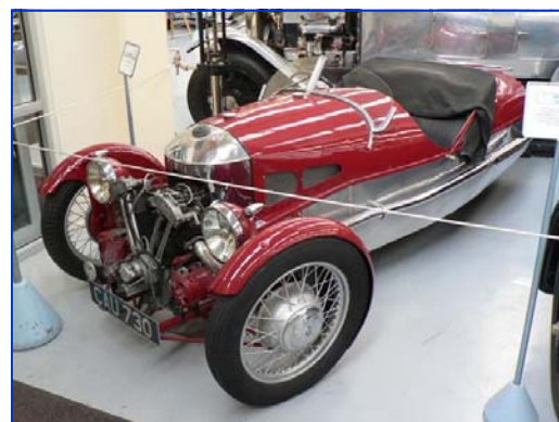
1935 Morgan Super Sports Barrel Back with an Air Cooled Matchless MKII - Twin
