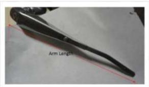
Figure 3. The Bayonet Style Wiper Clip and Wiper Arm. Note the flatter arm without the wrist bend.
