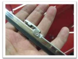
Figure 7. The 10" Holden Wiper blade with Bayonet Style Clip. Note Nylon spacer.
