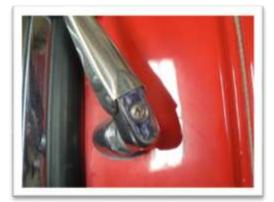
Figure 4. Pressure Key Tightening Screw
